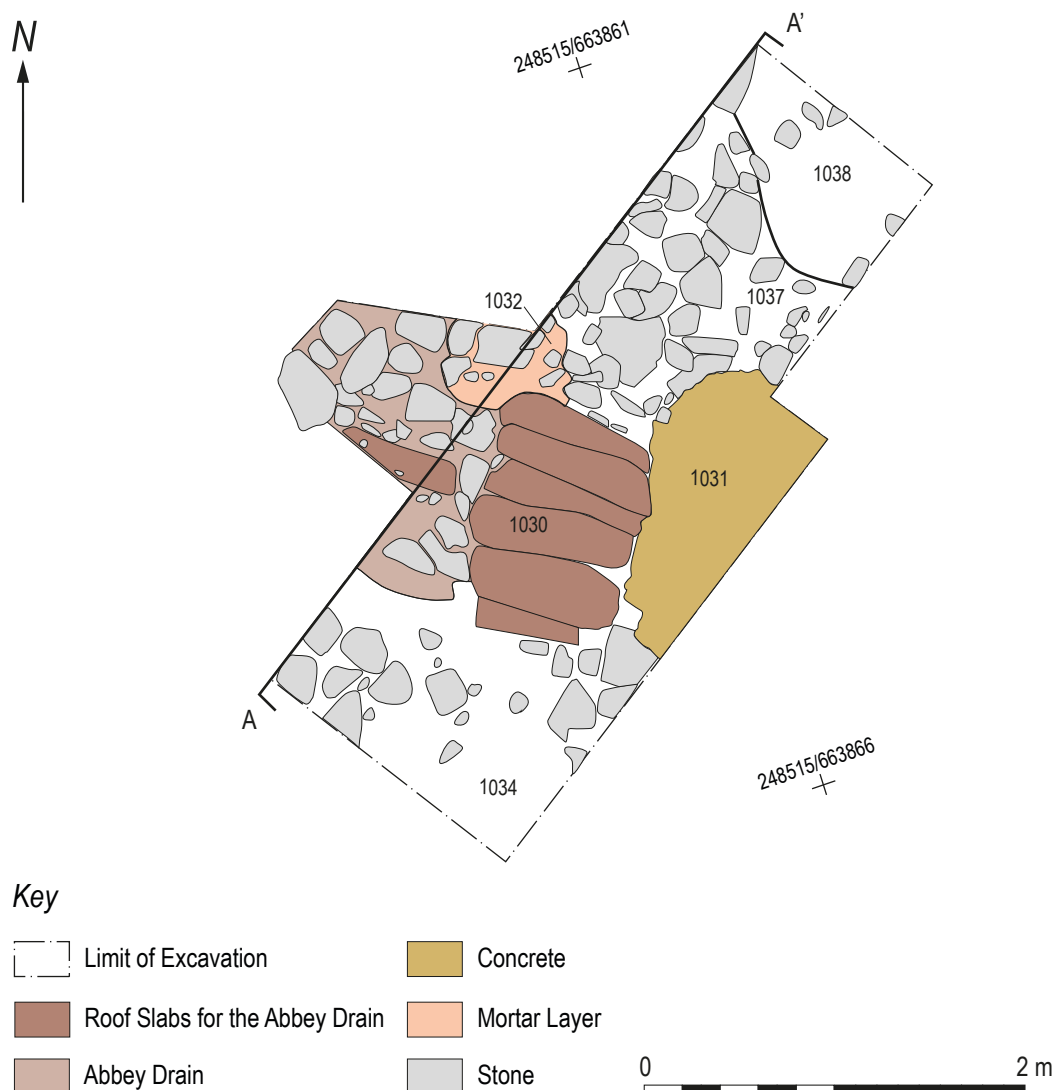
Figure 6: Plan of stone roof slabs 1030 of the Abbey Drain and concrete roof 1031 in MST
